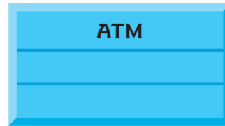
Fig. 25.6 | Representing a class in the UML using a class diagram.
